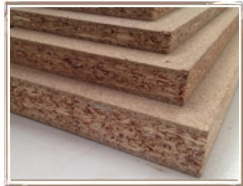
Particle board is the lightest board in fiber boards and with less strength to MDF board and other hard woods. Moreover, particle board will expand easily when exposed to the moistness. However, particle board is popular for interior usage as it has light weight, cheap and easy to move. In addition, particle board is environmental-friendly as no hard woods in the forest shall be cut down.
