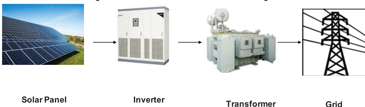
Figure 2-8: Power Generation from Solar Power Diagram
